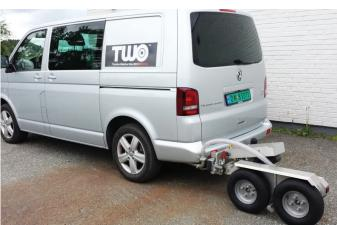
Friction meter using precise weight values for definition of friction. Friction meter additional equipment that provides exact local knowledge.
