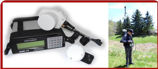
GEM Overhauser Magnetometer system. It can be configured with an additional sensor for simultaneous gradiometer readings, walking mode, gps
