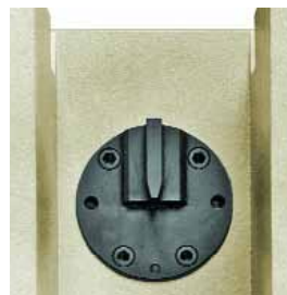
Fig. 6. View of the Charpy striker from the pendulum head.
