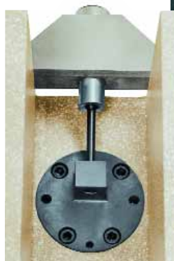
Fig. 10. View of the tension impact striker from the pendulum head. The sample is threaded into the 'striker' and the holding bar at the back of the pendulum head.
