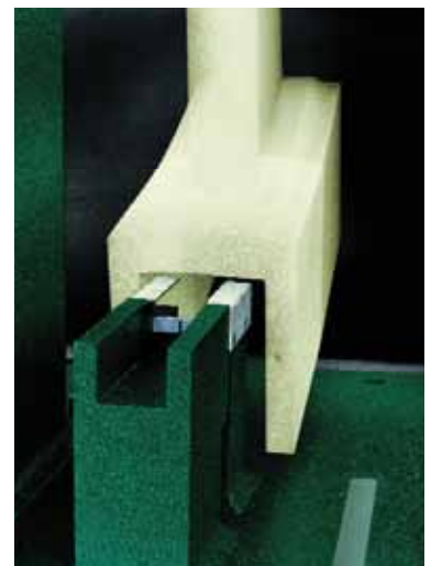
Fig. 5. Close up of Charpy set-up just prior to impact.
