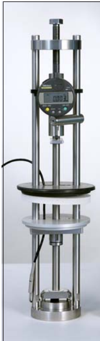
The test rig in the Freezer ET 03 adapted for Low Temperature compression set.
